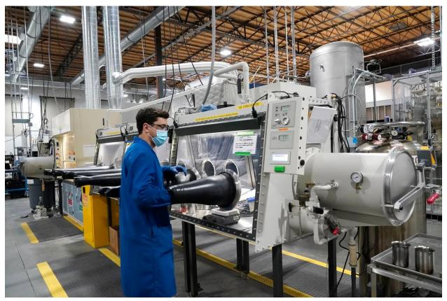
Test engineer Jacob Wilcox pulled his arm out of a glove box used for processing sodium at TerraPower in Everett, Wash. The company, of which Bill Gates is founder and chairman, is developing and building small nuclear reactors. ELAINE THOMPSON/ASSOCIATED PRESS
