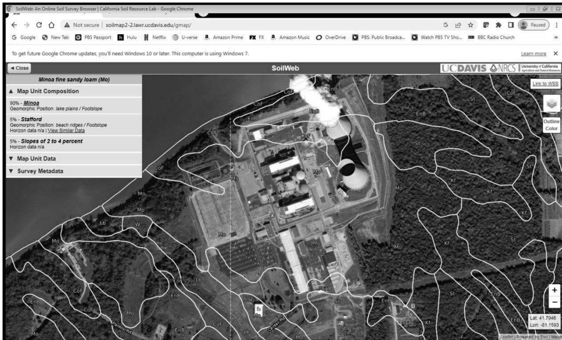
Figure 3: The soils of the area pf the Perry Plant. Source: University of California Davis web soil survey site, http://soilmap2-2.lawr.ucdavis.edu/gmap/
